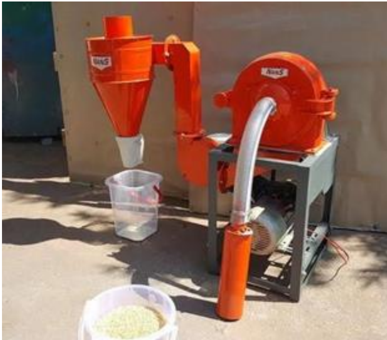
Hammer Millet Milling Machine (Capacity: 250 – 300 Kg/hr)
